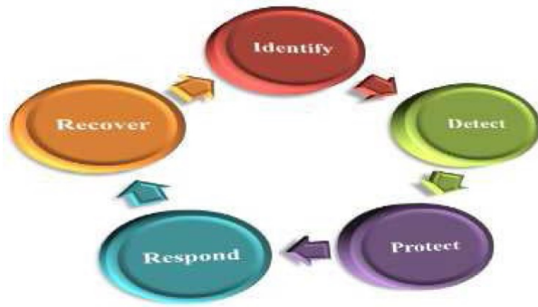
Figure 2. The five main functions of cyber security framework.
